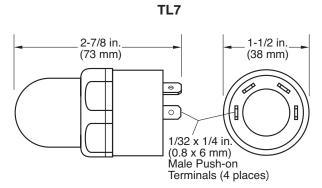
**Mounting Hole:** 1-1/8 in. (29 mm) diameter **Maximum Panel Thickness:** 1/4 in. (6 mm)
